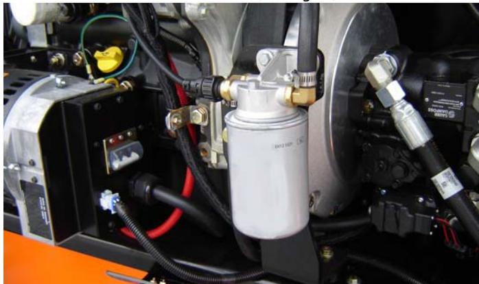
Lube Point(s) - Replaceable Element
