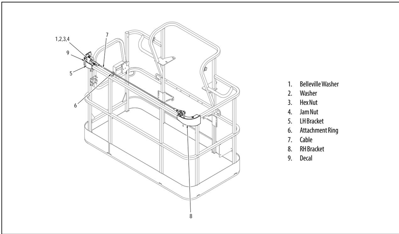
**Figure 6-2. Bolt-On External Fall Arrest System**
