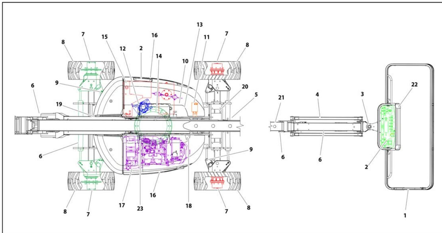
Figure 2-5. Daily Walk-Around Inspection Diagram - GM 3.0L
