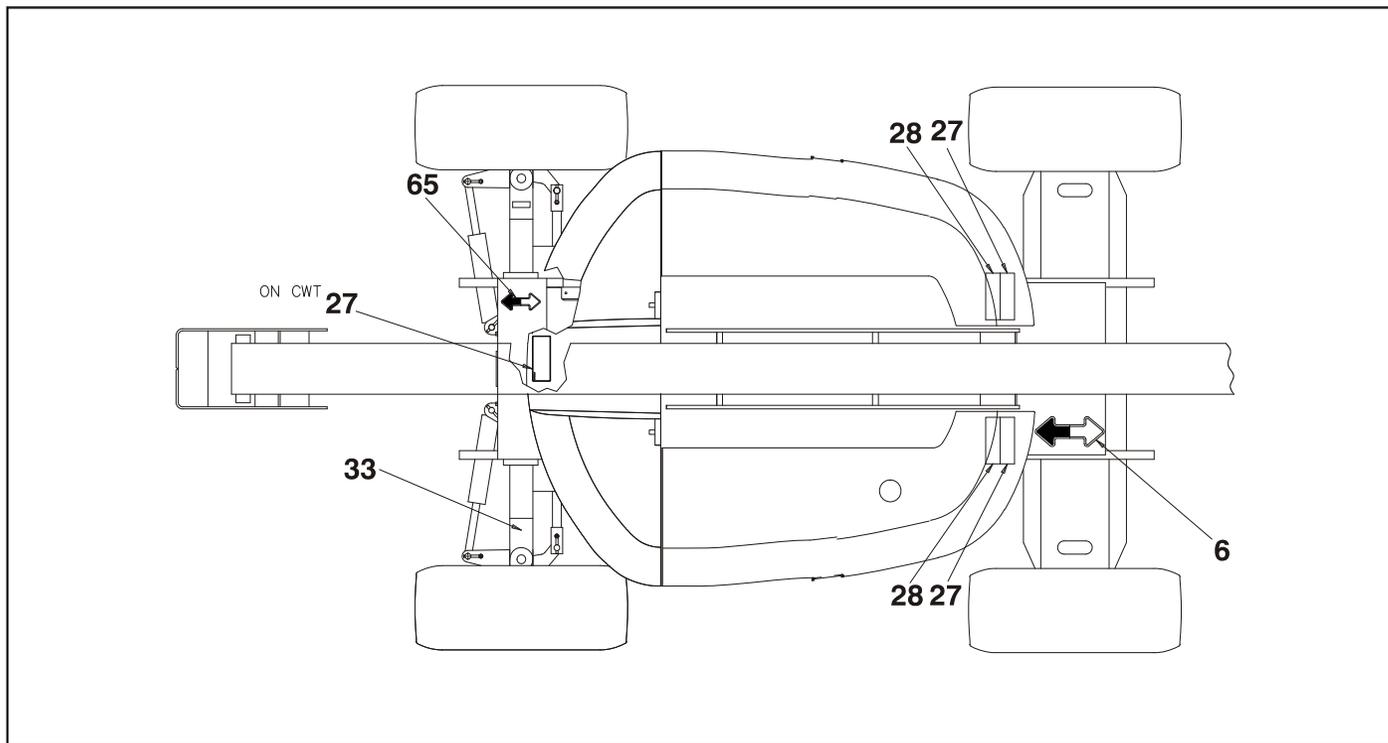
**Figure 4-14. 600A & 600AJ Decal Installation - Sheet 4 of 4**
