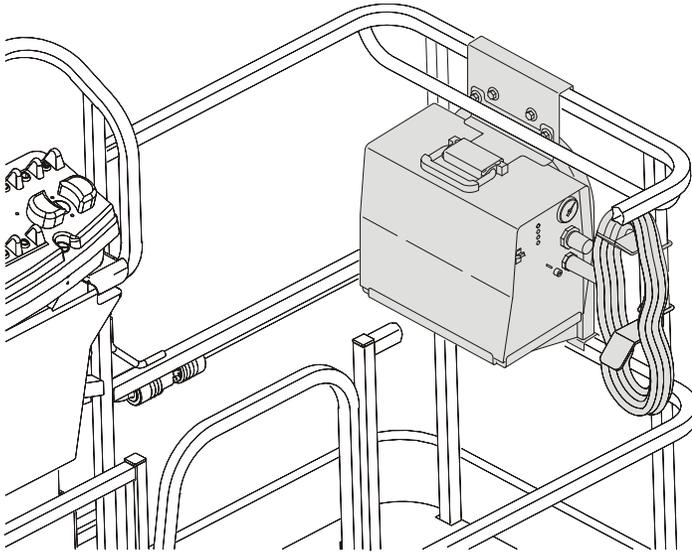
SkyCutter™ is capable of cutting up to a thickness of 3/8" metal. It can produce 27 A at 92 VDC at 35% duty cycle or 14 A at 92 VDC at 60% duty cycle. It receives power from the SkyPower™ system.
