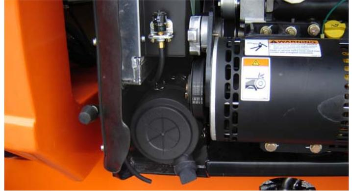
Lube Point(s) - Replaceable Element
