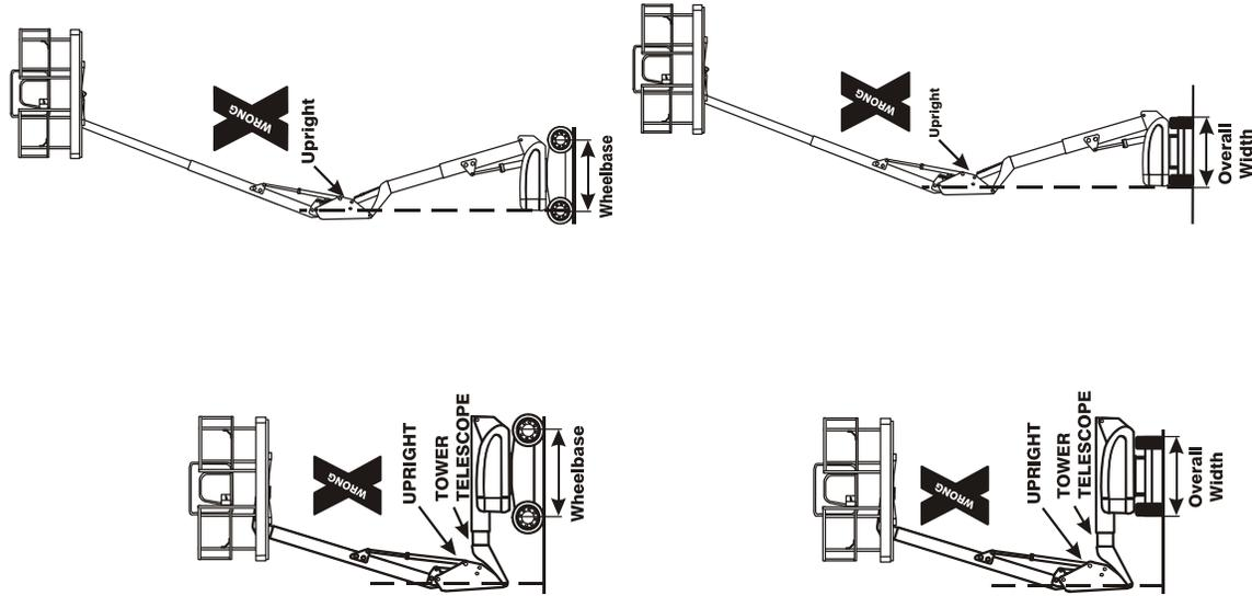
Figure 4-7. Boom Upright Positioning - Sheet 2 of 2
