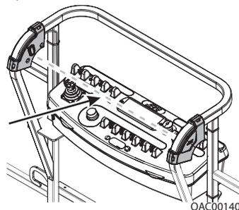
Operator passes through path of sensor beam.
