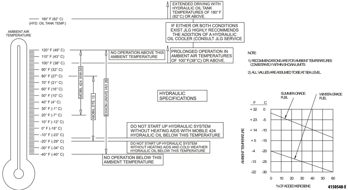
Figure 7-3. Engine Operating Temperature Specifications - Deutz - Sheet 2 of 2
