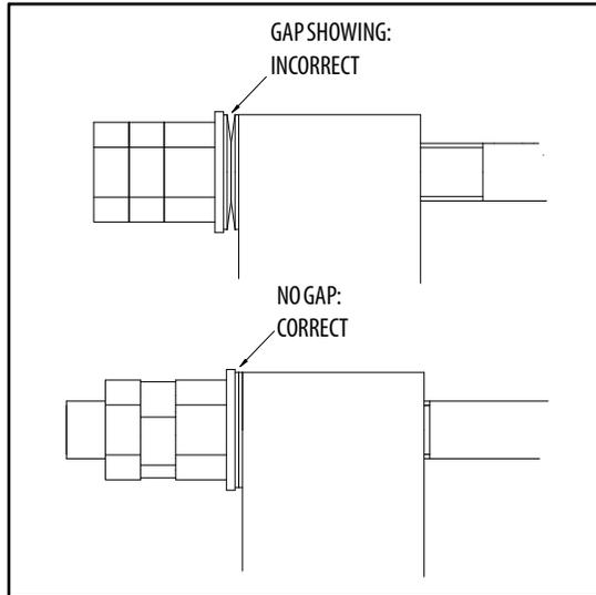
**Figure 6-1. Bolt-On External Fall Arrest Cable Tension**
