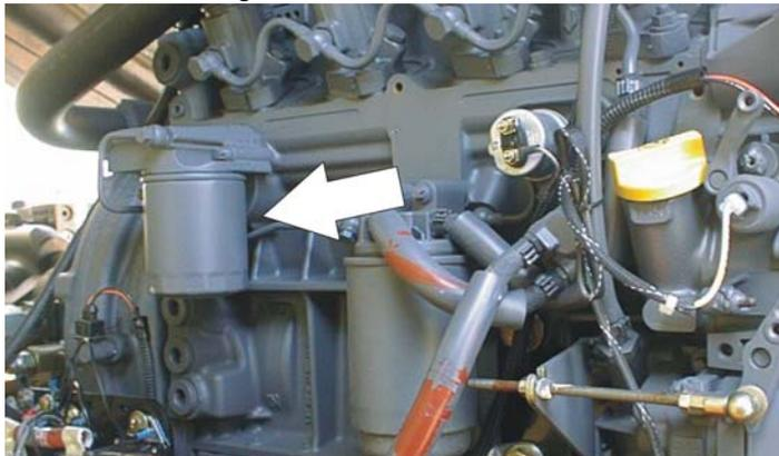
Lube Point(s) - Fill Cap/Spin-on Element
