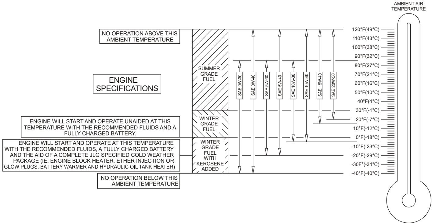
Figure 7-2. Engine Operating Temperature Specifications - Deutz - Sheet 1 of 2
