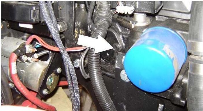
Lube Point(s) - Fill Cap/Spin-on Element
