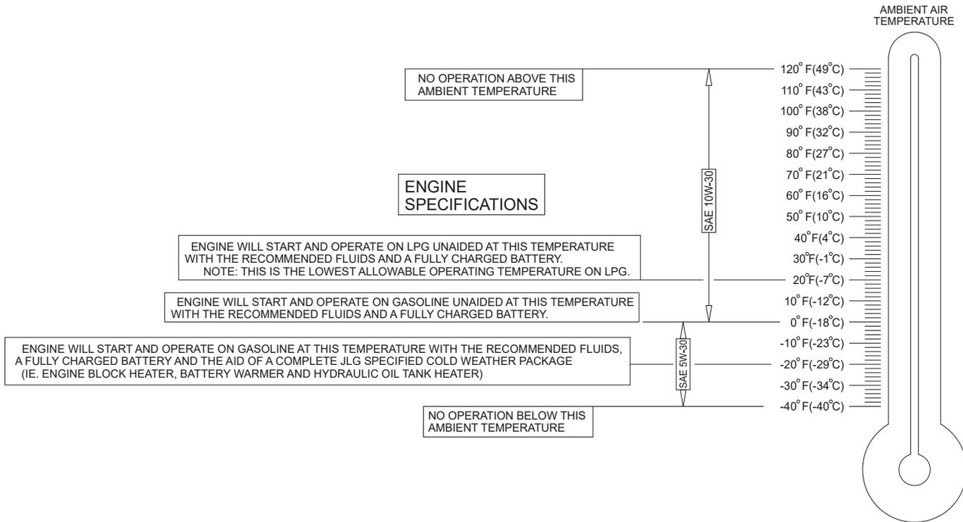
Figure 7-4. Engine Operating Temperature Specifications - GM - Sheet 1 of 2
