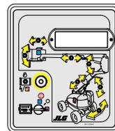
2. Open hand valve on LP gas supply tank by turning counter-clockwise.
