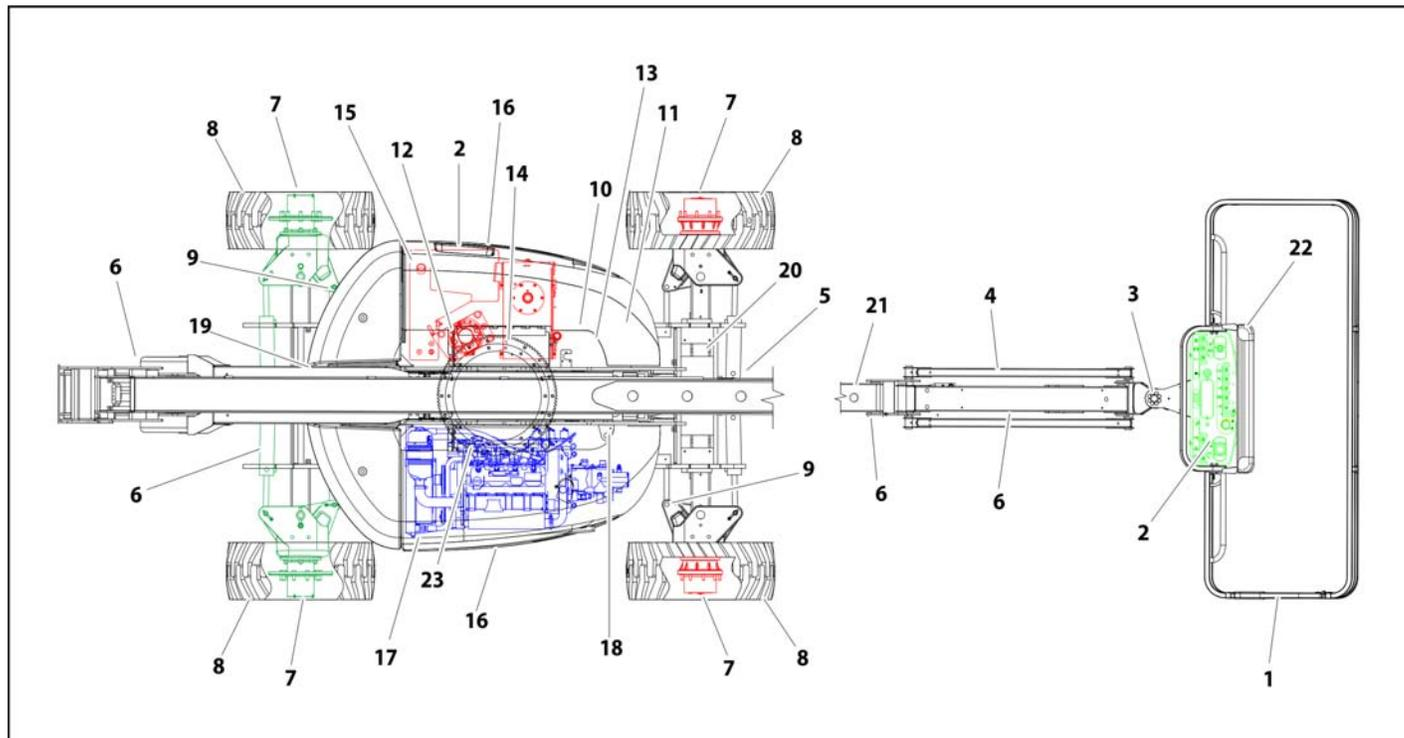
Figure 2-3. Daily Walk-Around Inspection Diagram - Deutz D2011L04
