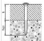
Nail Length = Embedment + Fastened Material Thickness
