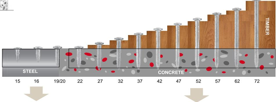
12mm into STEEL (Steel to steel Fastening)
