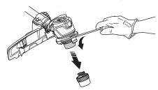
Remove the nut holding the trimmer head and the drive disc.
