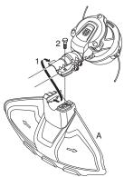
Hang the trimmer guard on the hook on the plate holder (1). Bend the guard around the shaft and tighten it with the bolt (2) on the opposite side of the
