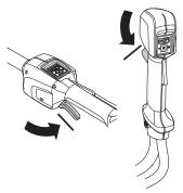
Press the power trigger and make sure it returns to its original position when you release it.
