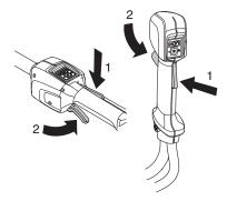
Make sure the power trigger is locked when the power trigger lock is in its original position.
