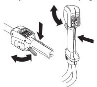
See instructions under the heading Start. Start the machine and apply full power. Release the power trigger and check that the cutting attachment stops and remain at a standstill.
