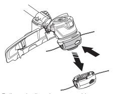
· Pull out the line chute assembly.
