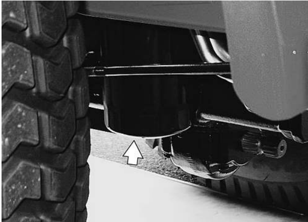
Figure 57 - Hydraulic Oil Filter
