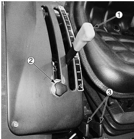
Figure 34 - Hydraulic Lift System Control
