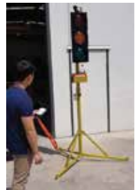
The lantern will start in test mode with nothing illuminated
