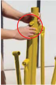
Pull spring pin to release leg
