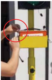
Lock latches to secure battery box
