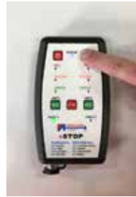
Switch to operation mode by holding the activation button for 5 seconds
