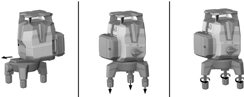
1. Remove the base plate by pulling it forward and clear of the device.
