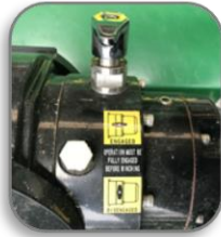
Winch handle in engaged position
