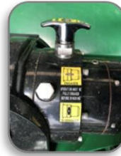
Winch handle in disengaged (free spool) position
