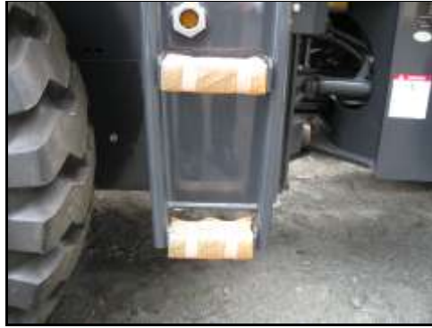
Vertical distance between step 1 and step 2 on RHS.
