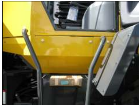
Hand rails a continuation of stiles on LHS.
