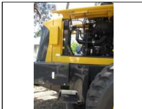
Rear maintenance step, no guard railing.
