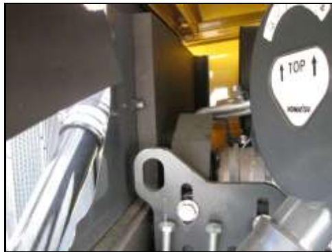
Air conditioning compressor belt pulley.
