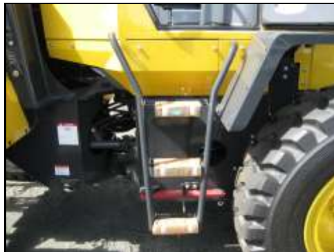
Tread heights and widths non-uniform on LHS step ladder.
