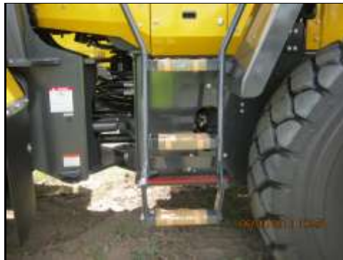
Vertical distance handrails commence above ground on LHS.
