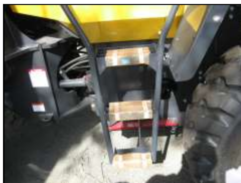
Clearance between step 3 on LHS and rear mud guard.
