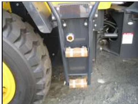
Tread heights and widths non-uniform on RHS step ladder.
