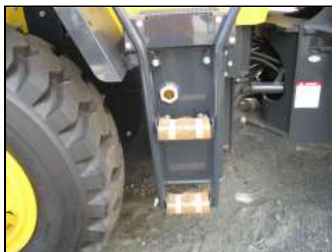
Non-uniform vertical rung distance on RHS step ladder.
