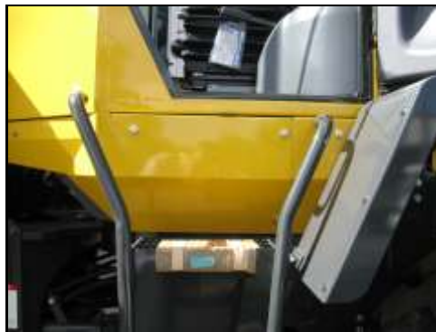
Top tread on LHS is below cabin floor landing.
