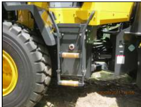
Vertical distance handrails commence above ground on RHS
