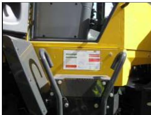
Hand rails a continuation of stiles on RHS.
