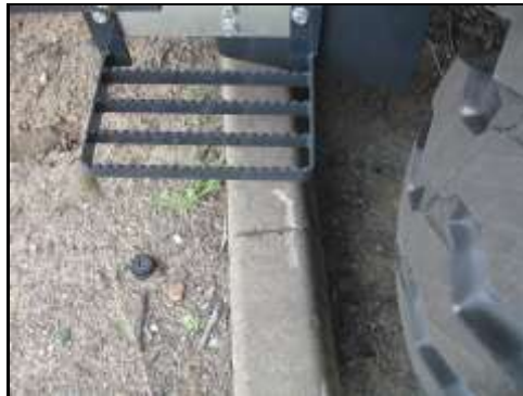
Clearance between rear maintenance step and tyre.
