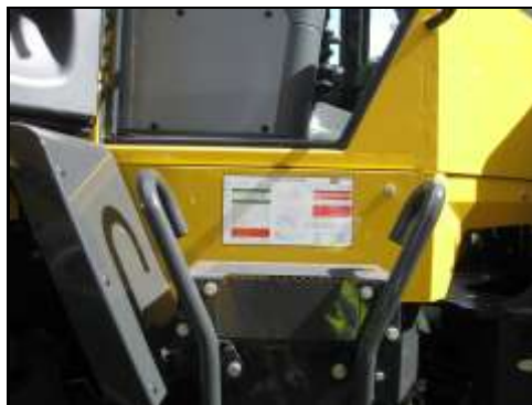
Top tread on RHS is below cabin floor landing.
