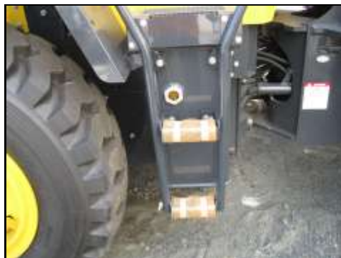
Clearance between step 3 on RHS and rear mud guard.
