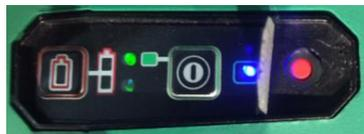
**STEP 4:** Once turned on you will see the two **'Orange'** fault lights flashing. To reset these hold down the 'Battery Indicator' button and the (now exposed) **'RED'** service button together for approx. 10 seconds at which point the **'Orange'** lights will stop flashing, and the gun is reset
