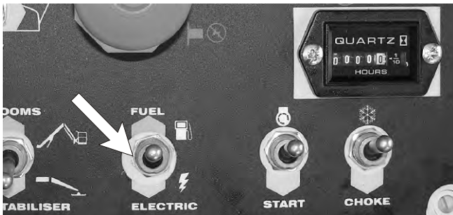
Figure 11.2.1 - Fuel / Electric Switch
