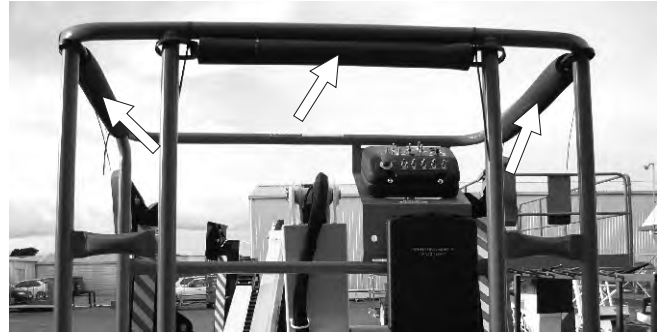
Figure 7.17 - Platform Gravity Gates
