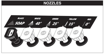
The four color-coded quick connect nozzles provide a wide array of spray widths from  $0^{\circ}$  to  $40^{\circ}$  and are easily accessible when placed in the convenient rubber nozzle holder, which is provided on the front of the machine.
