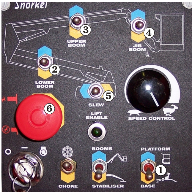
Figure 7.22 - Ground Control Switches
