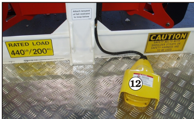
Upper Controls Foot Switch
