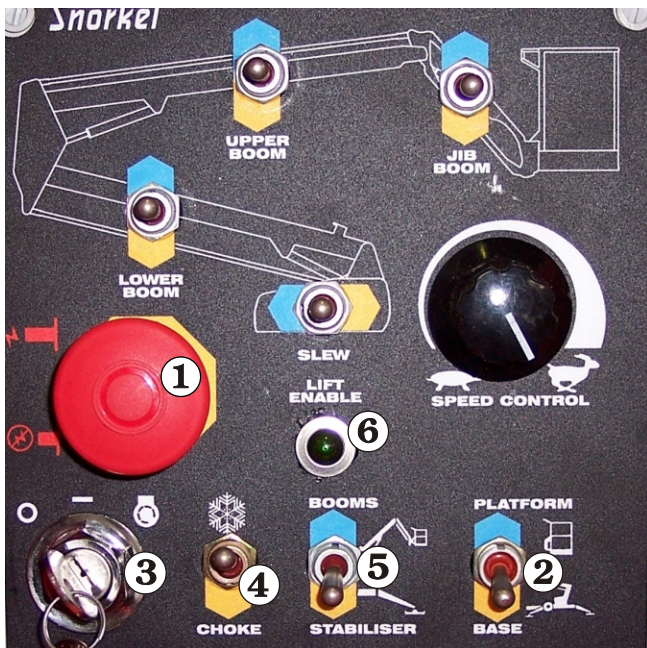
Figure 8.3 - Ground Control Box Starting
