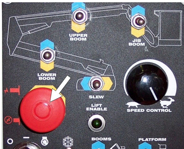
Figure 2.1 - Emergency Stop Switch at Ground Control Box
