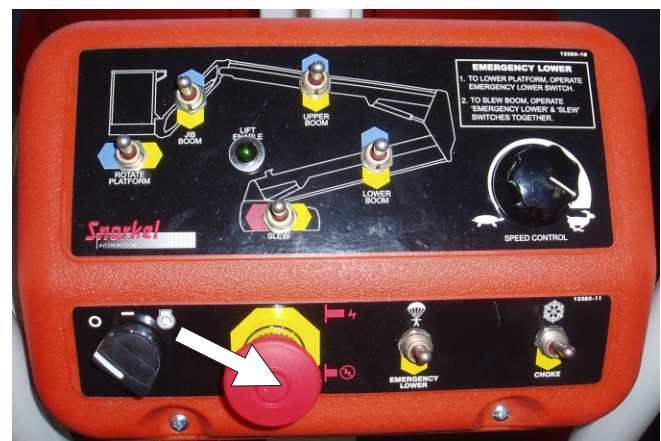
Figure 8.2 - Platform Control Box Emergency Stop Switch Location.
