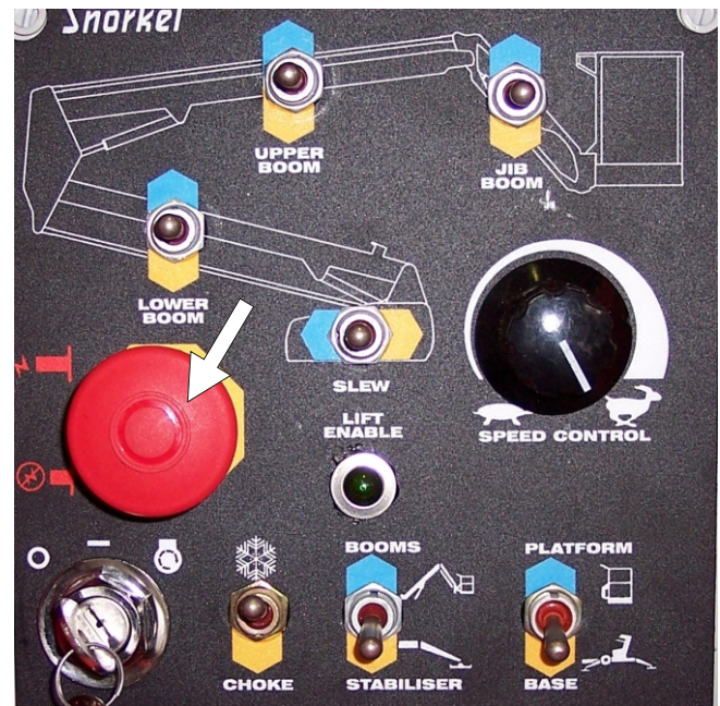
Figure 8.1 - Ground Control Box Emergency Stop Switch Location.
