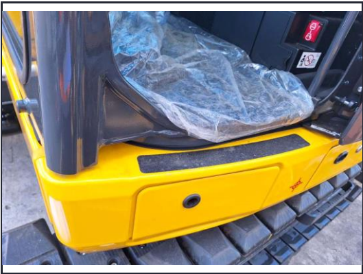
Anti-slip floor profile installed.
