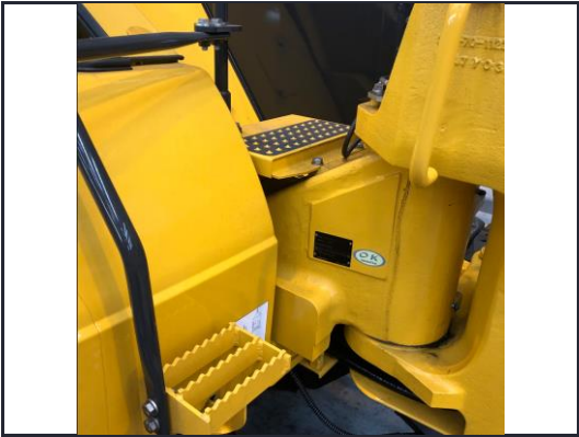
Rung step and maintenance platform.
