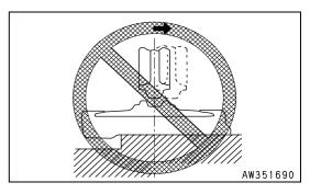
• If the machine is turned in this condition, the rubber shoe will come off.
