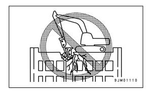
When carrying out demolition work, do not carry out demolition above your head. There is a hazard of broken parts falling or of the building collapsing and causing serious injury or property damage.
