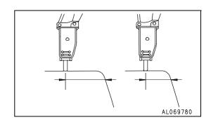
The direction of penetration of the chisel and the direction of the breaker body will gradually move out of line with each other, so always adjust the bucket cylinder to keep them aligned.
