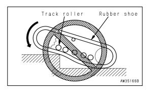
6. Furthermore, if the machine travels in reverse, a gap is formed between the track roller, idler, and rubber shoe.
