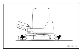
Open dirt cover (2) fully and secure it in position.
