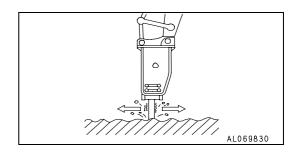
Holding the chisel horizontal or pointed up when carrying out impacting operations
