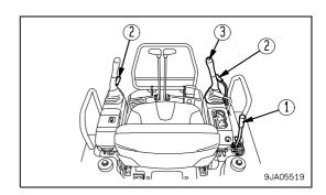
Pull fuel control lever (1) from low idling (position A) to midway position (B) between full speed and low idling to raise the engine speed to a mid-range speed, then run under no load for approx. 5 minutes.
