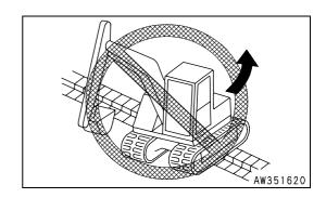
When traveling in reverse up a slope, do not turn when moving from flat ground onto the slope.
