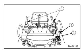
Check the safety lock lever (1) is at the LOCK position (L).
