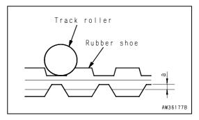
If the lug wears and the steel cord inside the shoe is exposed for two links or more, replace with a new part.
