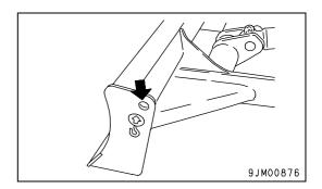
8. Pass the wire rope through the bracket on the boom (see diagram on right).
