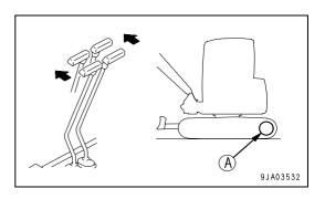
• When the sprocket (A) is at the front of the machine. Pull levers (3) backward slowly to move the machine off.
