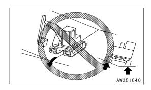
4. If the machine is operated as explained in 1 to 3 above, the rubber shoes is slackened. Do not steer the machine in the positions shown in the figure.
