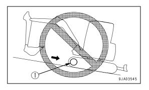
2. When traveling up a steep hill of more than 15°, set the work equipment to the posture shown in the diagram on the right.
