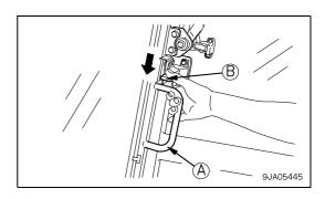
4. Grip left and right knobs (A) and pull the front window up diagonally.
