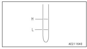
5. If the oil is above the H mark, drain the excess engine oil from drain plug (P), and check the oil level again.
