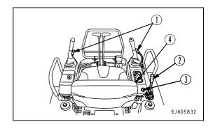
Check the safety lock lever (1) is at the LOCK position (L).
