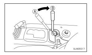
2. Set safety lock lever (2) to the FREE position, and raise the bucket from the ground.
