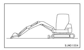
4. Set the safety lock lever to the LOCK position and stop the engine.
