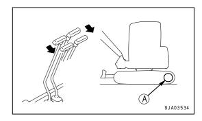
• When the sprocket (A) is at the front of the machine. Push levers (3) forward slowly to move the machine off.
