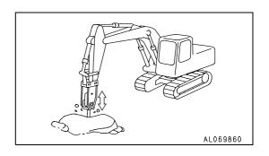
Extending the bucket cylinder fully and thrusting to raise the machine off the ground
