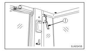
When escaping, break the window glass with hammer (1).
