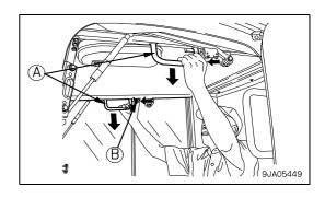
5. When the bottom of the window reaches the top of the bottom window, push left and right knobs (A) to the front, and push against left and right stoppers (C) to engage the lock.
