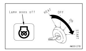
5. When the engine starts, release the key in starting switch (3). The key will return automatically to the ON position.
