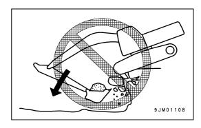
• To make it easier to escape if there is any problem, set the tracks at right angles to the road shoulder or cliff with the sprocket at the rear when carrying out operations.
