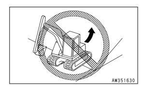
3. Avoid traveling along the edge of slopes or on rough groundwith the track on one side raised (with the machine tilting at anangle of more than approx. 10°) and with the track on the other side on flat ground. To avoid damage to the rubber shoes and road liners, travel with the tracks on both sides on flat ground.
