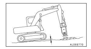
When applying continuous impact to the same impact surface, if the chisel does not penetrate or break the surface within 1 minute, change the point of impact and carry out breaking operations closer to the edge.
