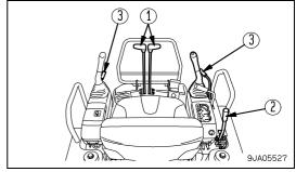
Put the left and right travel levers (1) in the NEUTRAL position, then stop the machine.
