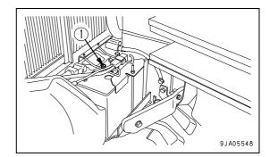
Use the diagram below for reference, and check if the electrolyte reaches the bottom of the sleeve.
