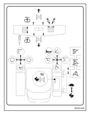
This left work equipment control lever (2) is used to operate the arm and upper structure.
