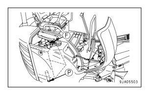
5. Extend the boom, arm, and bucket cylinder fully as shown in the diagram on the right, remove the oil filler cap, then install the cap and pressurize the inside of the tank.
