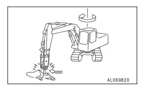
Moving the chisel while carrying out impacting operations
