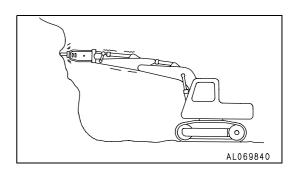
Twisting the chisel when it has penetrated the rock
