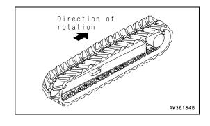
4. Fit a steel pipe in the rubber shoe, then rotate the sprocket again and fit the rubber shoe securely on the idler.
