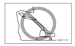
Do not excavate too deeply under the front of the machine. The ground under the machine may collapse and cause the machine to fall.
