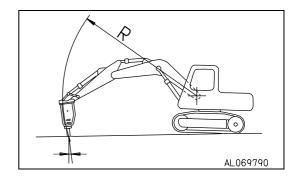
Always keep the chisel pressed against the impact surface properly to prevent using the impact force when there is no resistance.
