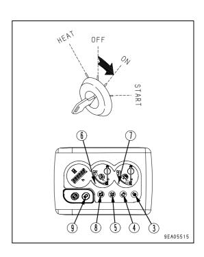
5. Press lamp switch (9) and check that the working lamp lights up. If it does not light up, there is probably a blown bulb or disconnection, so contact your Komatsu Utility Dealer for repairs.
