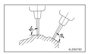
When applying impact, push the chisel against the impact surface and operate so that the chassis rises approx. 5 cm (2 in) off the ground. Do not let the machine come further off the ground than this amount.
