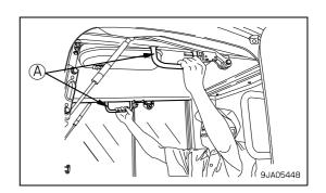
5. When it will move no further to the rear, push up knobs (A) to lock securely.
