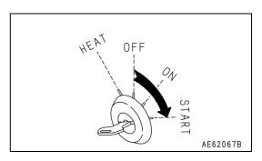
4. When the engine start, release the key in the starting switch (3). The key will return automatically to the ON position.
