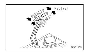
Lower fuel control lever (2) to low idling position (A) to reduce the engine speed.
