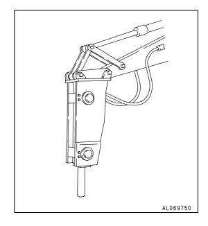
Keep the chisel pushed perpendicularly against the impact surface when carrying out breaking operations.
