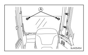
2. Install the lower window and push it down securely.
