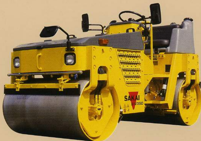
Double Drum Type SW350-1 2.8ton/1.2m (6,060 lbs/47")
